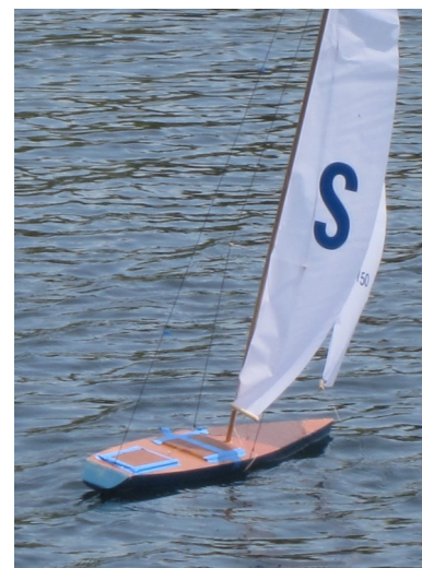
Model yacht "750 Racing Sparrow", being sailed by radio control,- 30inches long, built from scratch by Ian Sanderson
